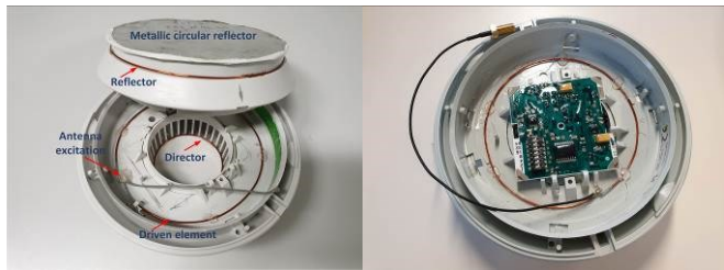
Fig. 5. Antenna parts integration in the smoke detector plastic shell.
