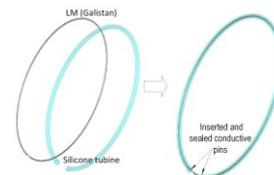
Fig. 2. LM based Loop antenna concept
