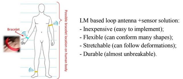
Fig. 1. LM based loop antenna integrated into the stretchable bracelet wearable sensor.
