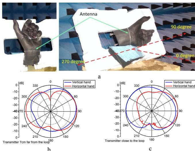
Sensor at 7cm distance from the loop antenna (at 868MHz)      Sensor is close the loop antenna (at 868MHz)
