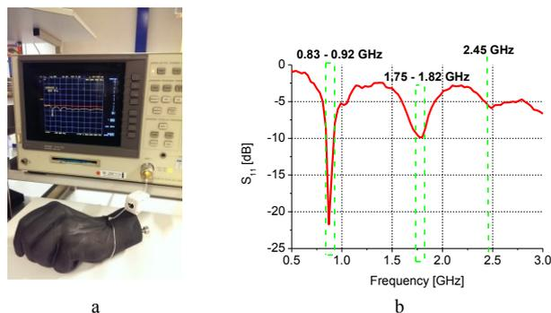
Fig. 6. Antenna S-parameter measurements
