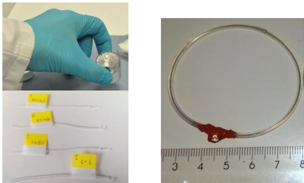
LM (Galistan) and silicone tubing Ready and sealed LM loop antenna
