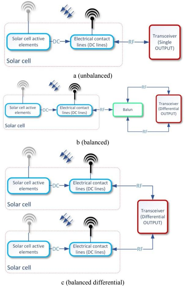
Fig. 2: General case block diagrams.
