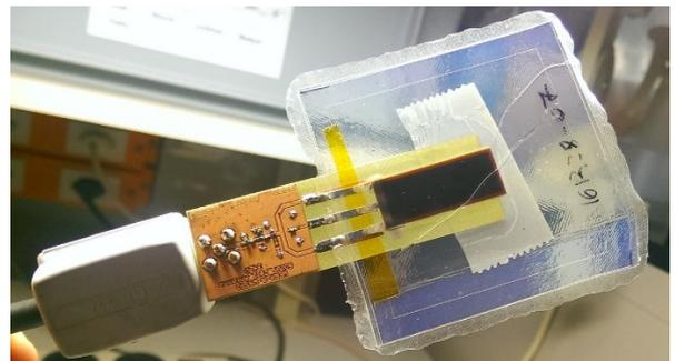
Fig. 5. Solar cell element antenna prototype.
