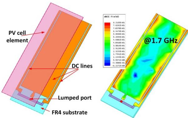
Fig. 3. PV cell antenna theoretical model and current distribution at resonance frequency.
