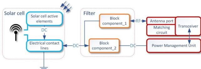
Fig. 1. Block diagram of the proposed antenna system solution.
