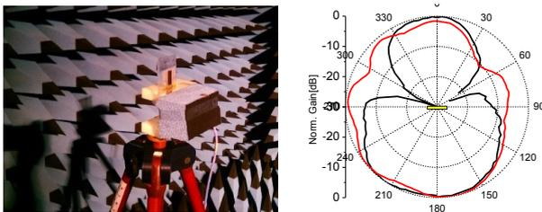
Fig. 7. Antenna under test: radiation pattern measurements @ 1.5GHz (CSEM anechoic chamber).
