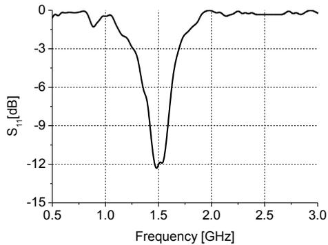
Fig. 6 Measured antenna S-parameter.
