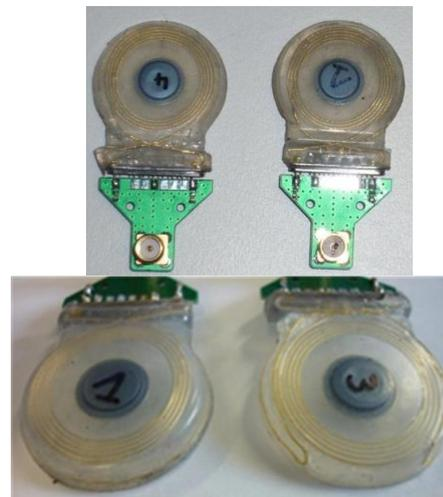
Fig. 5. Loop antennas in the silicone shell with matching circuit photos: circular loop antenna sample (left) and folded loop (right).
