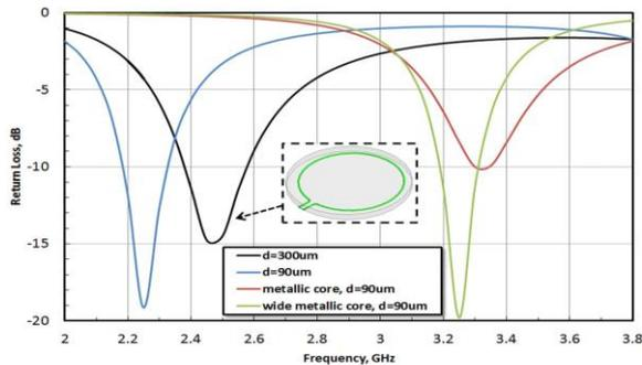
Fig. 3. Simulated performance characteristics for the integrated loop antenna
