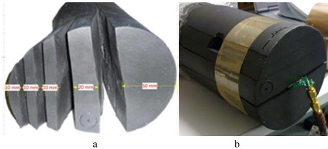
Fig. 6. Body tissue material prepared for antenna S-parameter measurements (a), antenna inside the material (b).
