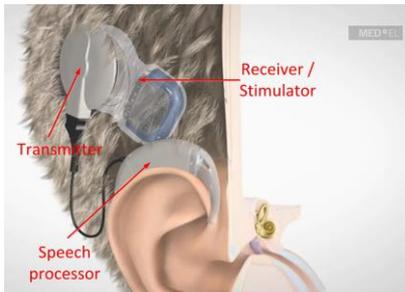
Fig. 1. Ear with cochlear implant drawing (picture is taken from MEDEL source [1])
