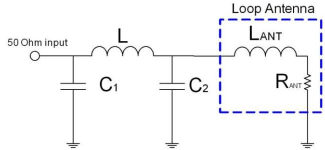
Fig. 4. Proposed lowpass PI matching network
