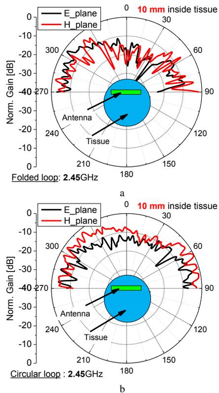
Fig. 9. Measured antenna radiation pattern at 2.45 GHz
