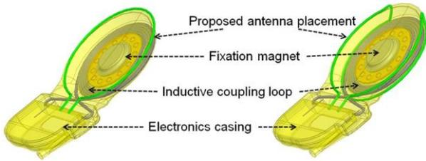
Fig. 2. Topology of the integrated loop antenna: circular loop antenna (left), folded loop antenna (right)
