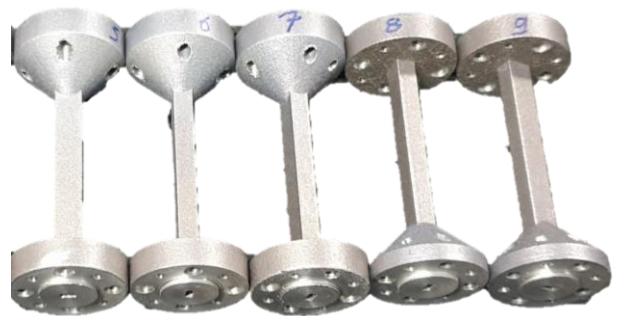
Fig. 4: 3D printed hollow WR-10 WG sections.
