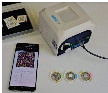
Figure 3: Chipless TAGs (short and long-range) reader developed at CSEM: a portable device for the measured parameter visualization, reader with integrated antenna and short-range chipless tags.
