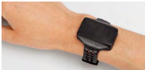
Figure 1: CSEM proprietary watch-like reflectance pulse oximeter device.
