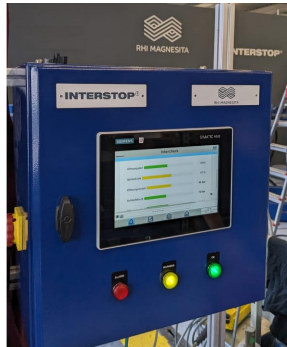
Figure 3: The Health Check Platform's operator-facing application makes relevant health indicators, virtual sensors, and sensor measurements accessible via HMI directly at the LPA or via browser anywhere within the steel mill's protected network and provides a feedback interface for experts' assessment of plate health.
