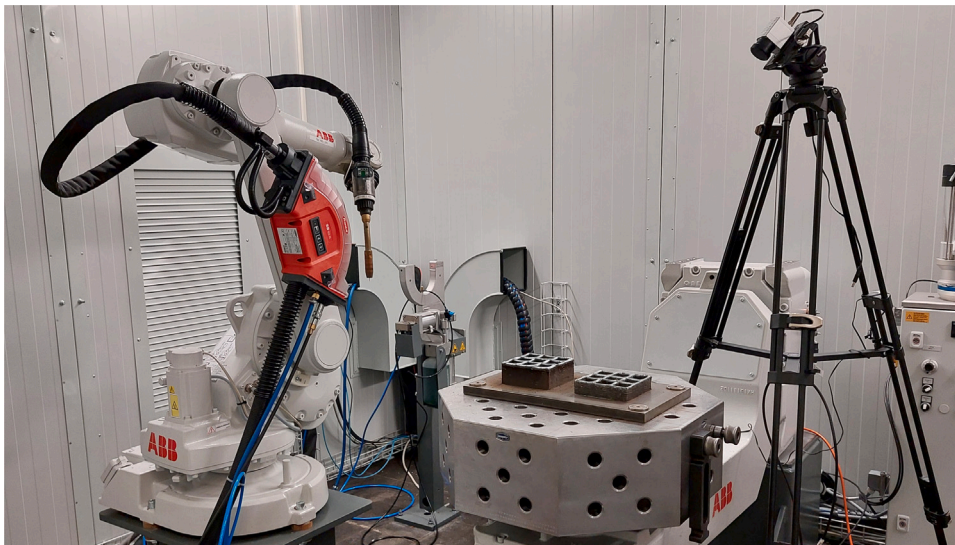
Fig. 4. The welding cell used for the experimental validation of the pipeline.
