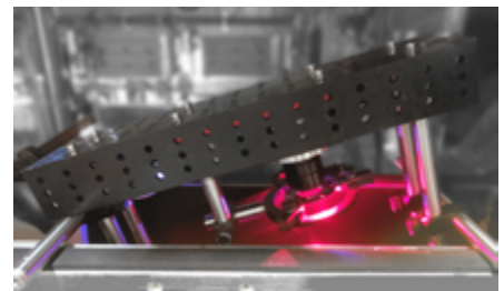
Figure 1: Optical system based on non-contact imaging measuring waste water quality.
