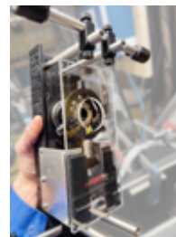
Figure 1: Optical system based on non-contact imaging measuring waste water quality.
