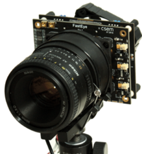
FastEye mounted with a 50 mm 1.8 f lens
