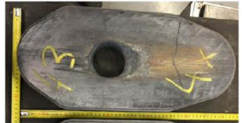
Worn out ladle gate plate
